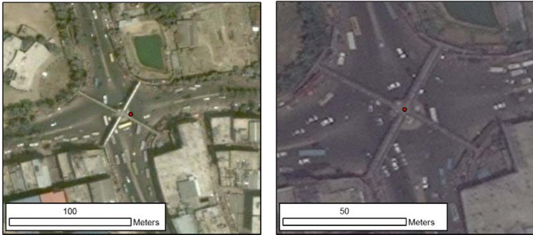
Figure 4. Misalignment of Bing aerial imagery in Bangladesh. The red dot indicates the same location displayed over Bing imagery at different zoom levels. (Left: smaller scale, right: larger scale)
